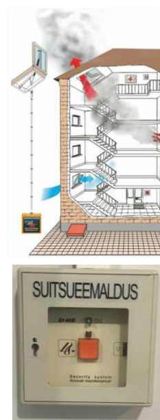
Image 8 Control button and smoke vents
